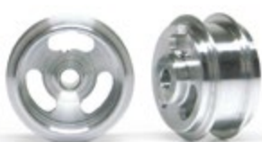
W15808215AF ex PA24-Alf Al ∅15.8 x 8.2 x 1.5mm wheels double shoulder M2 grub - 1.1g (2x)
